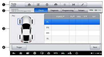
Figure 5-7 Sample Relearn Procedure for Indirect TPMS
