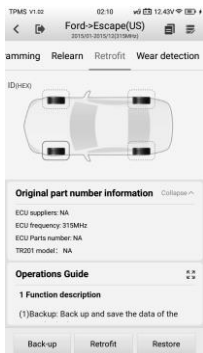
Figure 5-1 Sample TPMS Retrofit Screen
