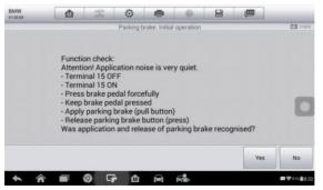
Figure 5-7 Sample Parking brake: Initial operation
