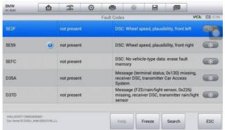
Figure 4-16 Sample DTC & FFD Screen
